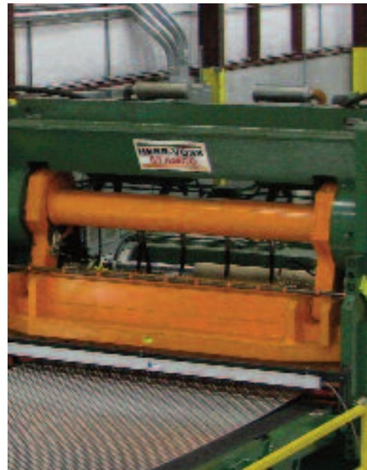
**[ RIGHT ]** The semi-bowtie blade of the downcut mechanical shear fires at 200 strokes per minute, will make a maximum of 60 cuts per minute and runs at a line speed up to 200 feet per minute. The top knife is adjustable for clearance.
