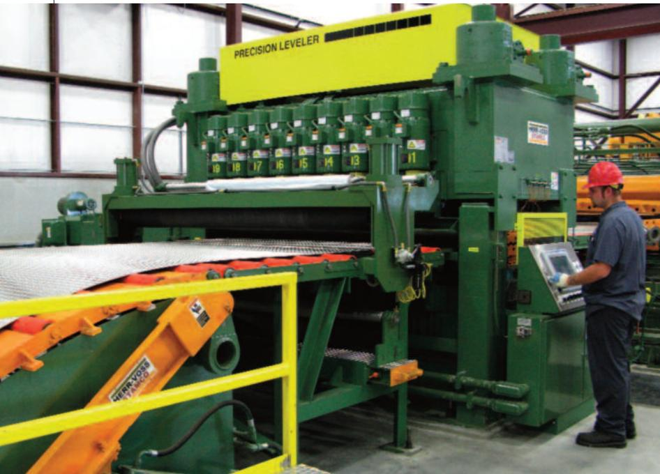
**[ LEFT ]** Line Operator Cody Henson at the controls of the precision roll leveler. The frame, hydraulics and 300-horsepower drive are typical for a leveler with 11 work rolls; this unit contains 17 rolls for deeper penetration and enhanced stress relief.
