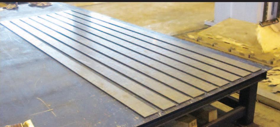
developing a process that would address not only the ability to produce stay-flat material but also overcome some of the shortfalls of other processes. Enhanced Leveling Technology creates flat material that stays flat by subjecting it to very severe and uniform bending work. This technique works materials longitudinally and through 100 percent of the material's width. "And by that work, mitigates non-uniform strains in two directions as well as the crossbow defect," Dias says.
