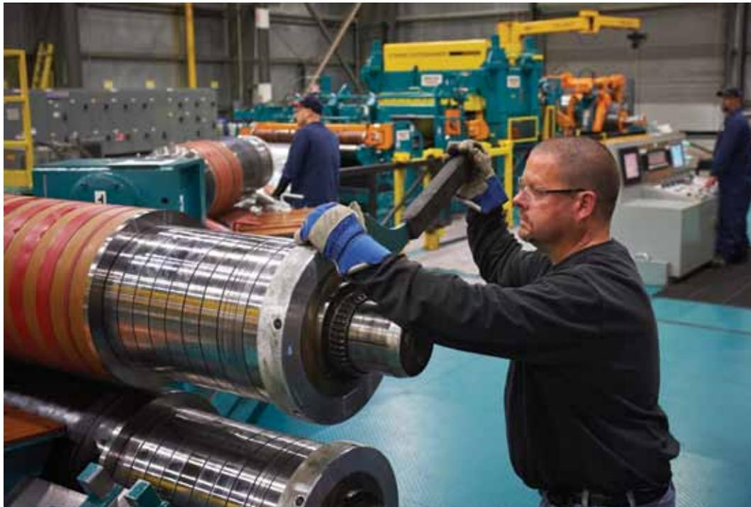
*A worker at Taylor Steel readies the tooling on the company's new high-strength slitting line. The arbors for the tooling are an oversized 12 inches in diameter to prevent deflection during the slitting process.*
