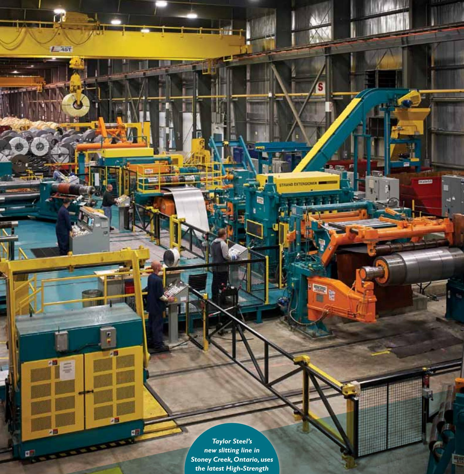
*Taylor Steel's new slitting line in Stoney Creek, Ontario, uses the latest High-Strength Slitting Technology from Herr-Voss Stamco. (Photos courtesy Taylor Steel)*
