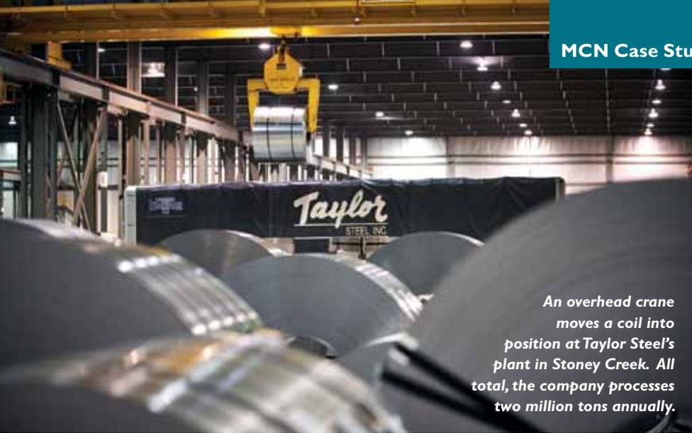
*An overhead crane moves a coil into position at Taylor Steel's plant in Stoney Creek. All total, the company processes two million tons annually.*
